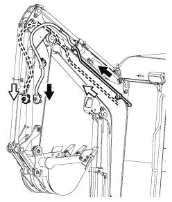
\* During single acting operation, the side shown by the black arrow is under high pressure.
