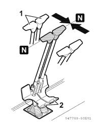
2. Move the engine speed control lever 3 or turn the engine speed control dial 3 to the IDLING position.
