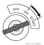
**3.** After the engine has started, release the starter switch key.
