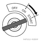
**4.** After the engine has started, release the starter switch key.
