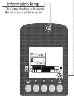
Information icon This icon is displayed to indicate the existence of information. Pressing the F4 switch allows checking of information details.
