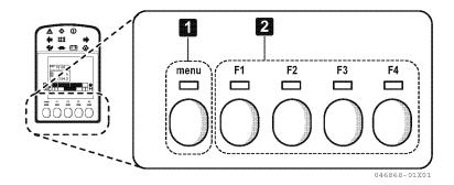
The function switches in the bottom part of the LCD monitor comprise 5 switches (a menu switch and F1 - F4 switches) and their functions change depending on the status of the machine or the screen currently displayed.
