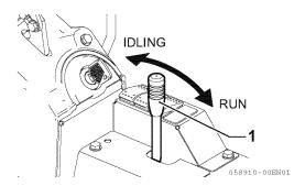
For the unit with the auto deceleration system, turn the engine speed control dial 1 to the "RUN" direction.
