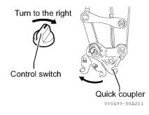
**7.** Only one of the bores allows the whole lock pin. Install the lock pin to that bore.
