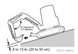
2. When climbing a slope, drive the machine with the implement positioned as shown in the right figure.
