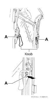
3. Lock the upper windshield housed under the ceiling securely with the right and left lock levers.
