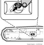
6. The tension can be adjusted until the clearance "a" is reduced to 0 in. (0 mm). If the tension is still loose after adjustment, the pin and the bush should be reversed or replaced because they are worn excessively. Ask your dealer to repair the track.
