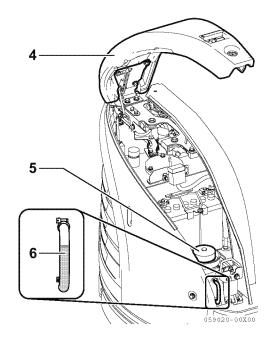
2. After refueling, securely retighten the fuel supply port cap, and close the bonnet B 4.
