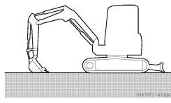
**2.** Lower the attachment onto the ground.
