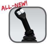
Single Control Joystick with boom functions, fork tilt and aux. line control, and also F-N-R shifting.
